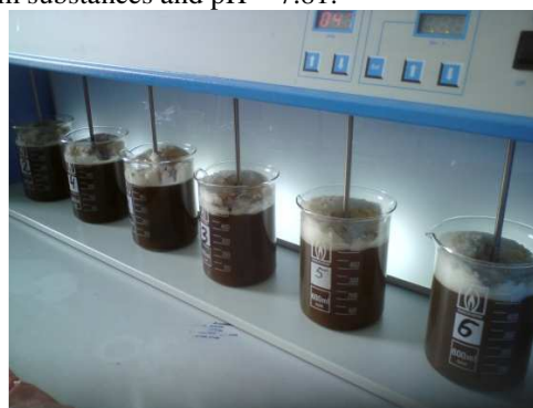
Fig.1 The test stand for the oxidation and coagulation of leachate from the landfill in Promnik
